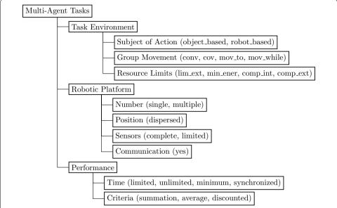
**Fig. 4** A graphical representation of *Balch* taxonomy (Balch 2002), with three axes: *Task Environment, Robotic Platform* and *Performance*. Where: coverage (*cov*), convergence (*conv*), movement from initial to final locations (*mov\_to*) or maintaining a configuration while moving (*mov\_while*), limited external resources (*lim\_ext*), minimum energy task (*min\_ener*), competition between team members for resources (*comp\_int*) and team competes with external agencies (*comp\_ext*)
