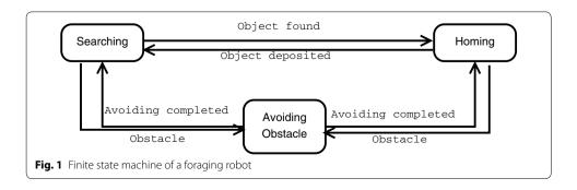
obstacle is encountered. The finish time of foraging is when all objects are located and transported to the home.
