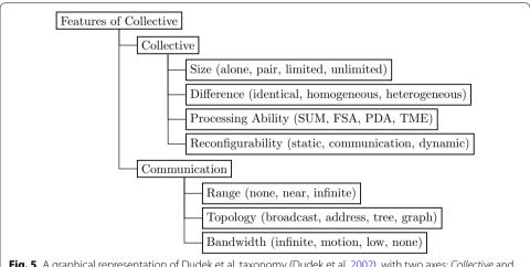
**Fig. 5** A graphical representation of Dudek et al. taxonomy (Dudek et al. 2002), with two axes: *Collective* and *communication*. Where: non-linear SUMmation unit (*SUM*), Finite State Automaton (*FSA*), Push-Down Automaton (*PDA*) or Turing Machine Equivalent (*TME*)
